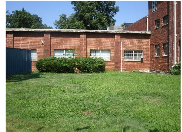
A rain garden can be installed south of the school to capture, treat, and infiltrate the stormwater runoff from the rooftops in that area. A preliminary soil assessment suggests that the soils have suitable drainage characteristics for green infrastructure.
